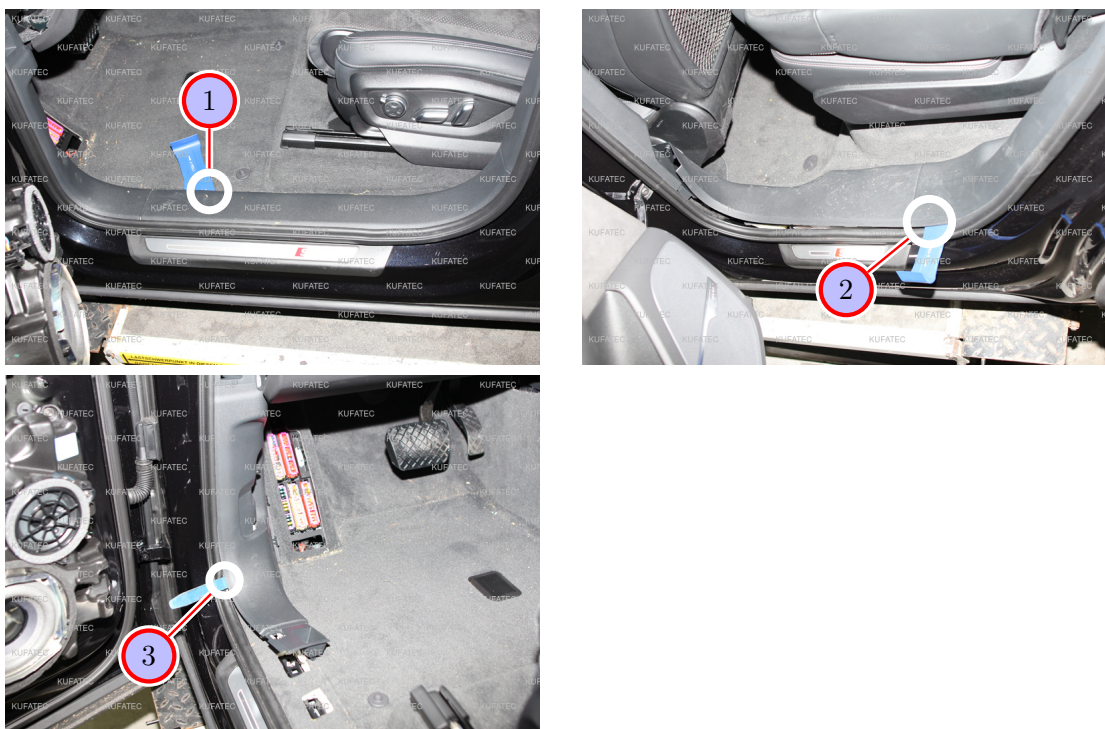
Figure 8: Removing trim panel driver's side
