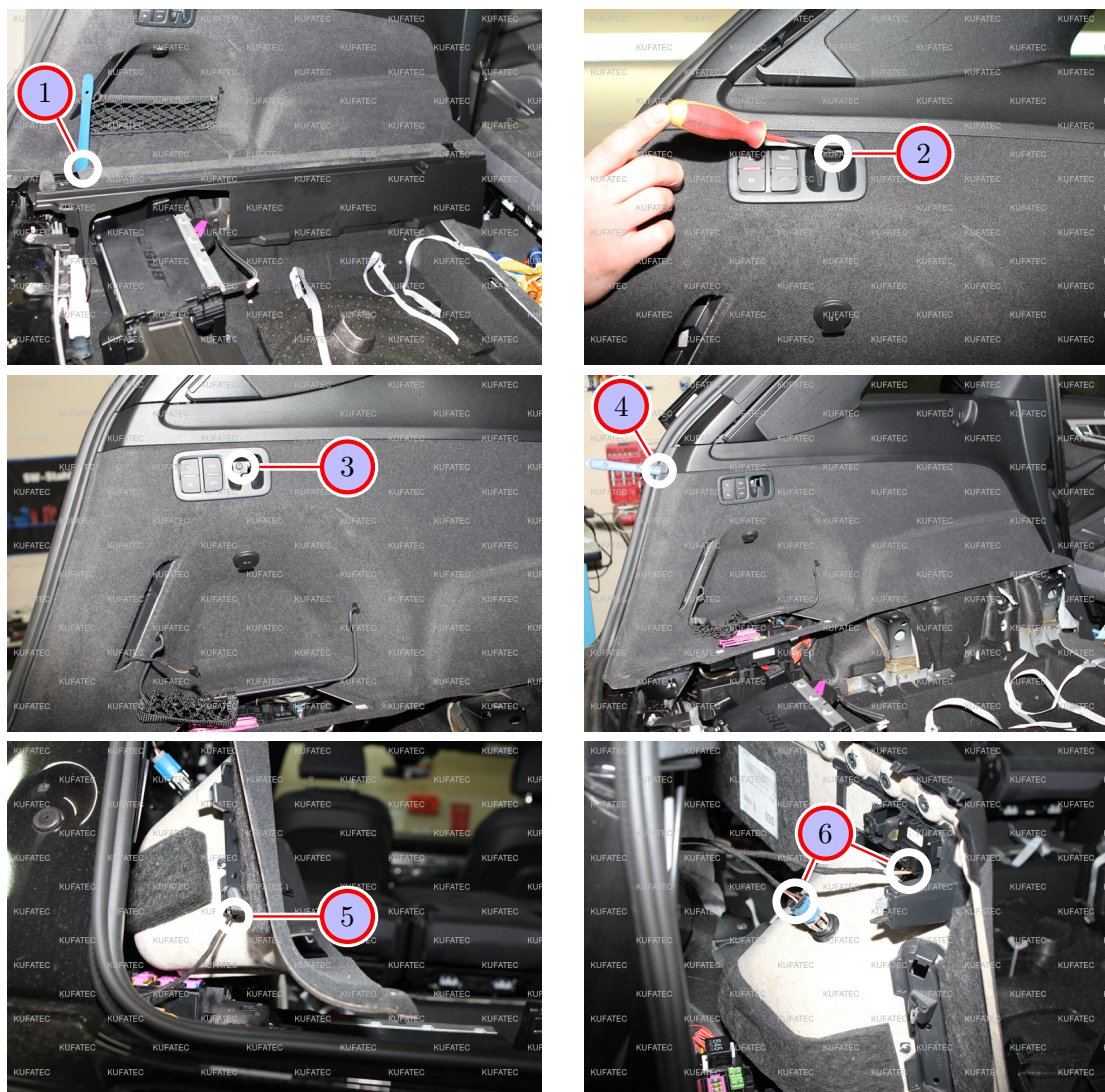
Figure 5: Disassembly left side covering trunk
